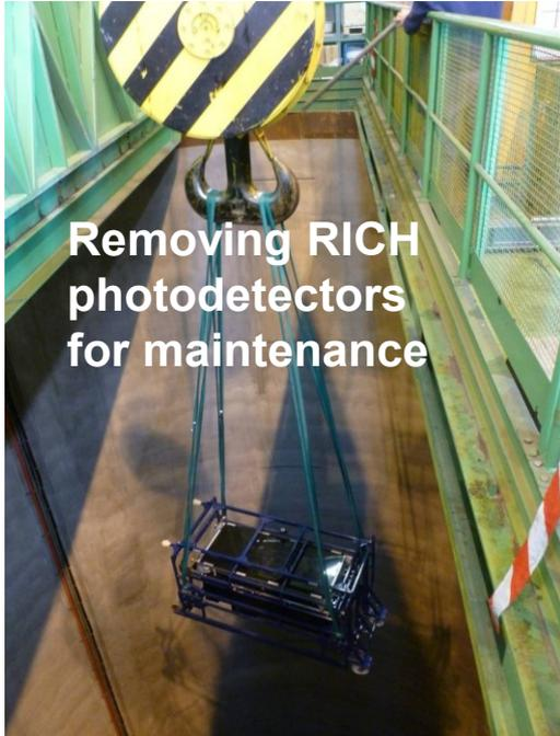
Removing RICH photodetectors for maintenance
