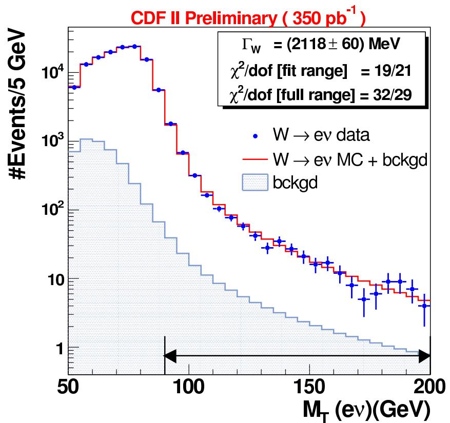
Result from CDF:  $\Gamma_W = 2.032 \pm 0.071 \text{ GeV}$  (=most precise single measurement)
