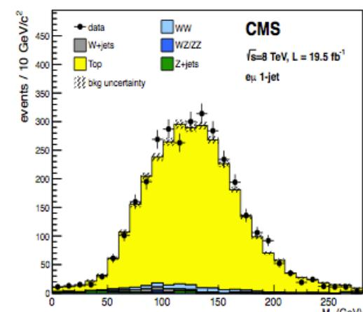
Figure 31:  $m_{\ell\ell}$  (left) and  $m_{T\ell\ell}$  (right) distributions in the 1-jet category for b-tagged events in different-flavor final state at the WW preselection level at  $\sqrt{s} = 8 \text{ TeV}$ . The uncertainty band includes the statistical and systematic uncertainty of all background processes.
