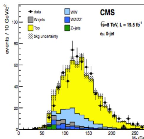
Figure 30:  $m_{\ell\ell}$  (left) and  $m_{T\ell\ell}$  (right) distributions in the 0-jet category for different-flavor final state at the WW preselection level at  $\sqrt{s} = 8 \text{ TeV}$ . The uncertainty band includes the statistical and systematic uncertainty of all background processes
