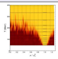
Left: Binder cumulant of the Polyakov loop as function of  $\mu$  and T. Right: Two dimensional projection of the Binder cumulant. Red colours indicated a value compatible with 0, while yellow corresponds to 2/3.
