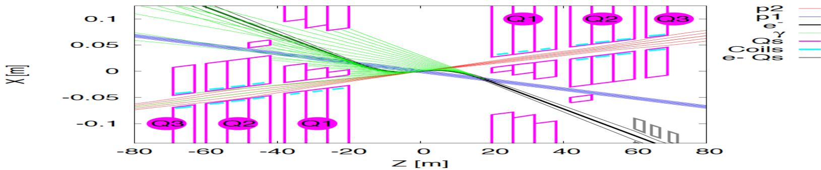
Tentative:  $\epsilon_p = 2\mu\text{m}$ ,  $\beta^* = 20\text{cm} \rightarrow \sigma_p = 3\mu\text{m} \approx \sigma_e$  matched!  $\epsilon_e = 5\mu\text{m} \dots$
