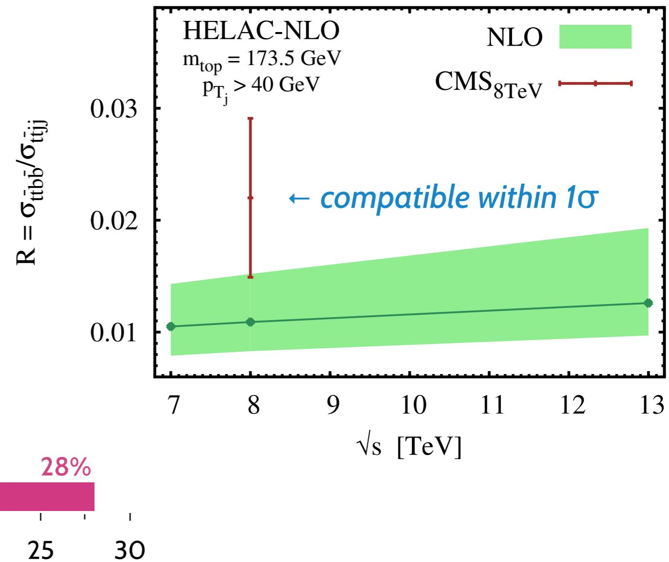
**Absolute  $\sigma_{ttjj}$ ,  $\sigma_{ttbb}$ ,  $\sigma_{ttbb}/\sigma_{ttjj}$ :** additional (b) jet  $p_T > 40$  GeV,  $|\eta| < 2.5$
