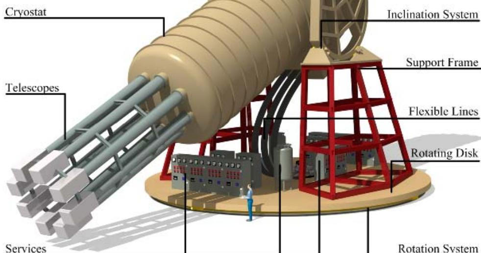
Magnetic length 20 m Total cryostat length 25 m
