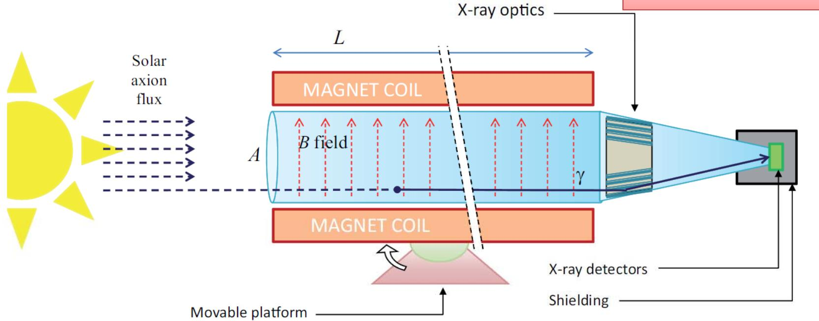
$$g_{a\gamma}^4 \propto \underbrace{b^{1/2} \epsilon^{-1}}_{\text{detectors}} \times \underbrace{a^{1/2} \epsilon_o^{-1}}_{\text{optics}} \underbrace{(BL)^2 A^{-1}}_{\text{magnet}} \times \underbrace{t^{-1/2}}_{\text{exposure}}$$
