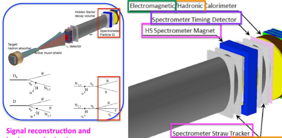
background rejection: warm magnet (LHCb) with 0.65Tm bending power; tracker (NA62) with horizontal straws and stereo angle
