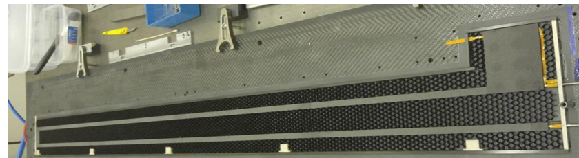
Stave being assembled. Carbon fibre honeycomb.
