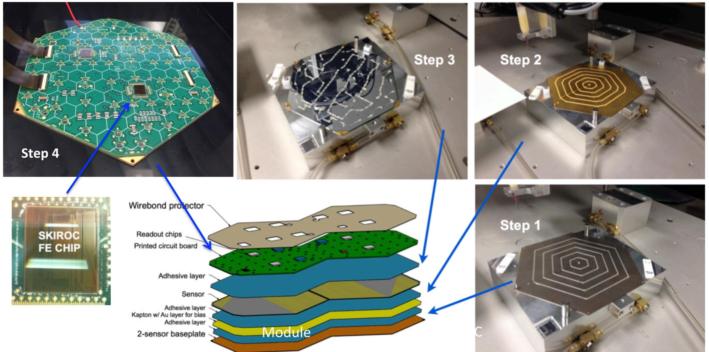
Successful module assembly for Fermilab test beam
