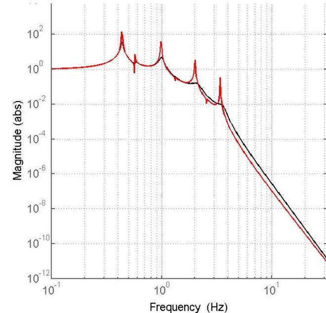
$$\left( \frac{x_{mass}}{x_{ground}} \right) \approx \frac{\omega_0^2}{(\omega_0^2 - \omega^2)}$$
