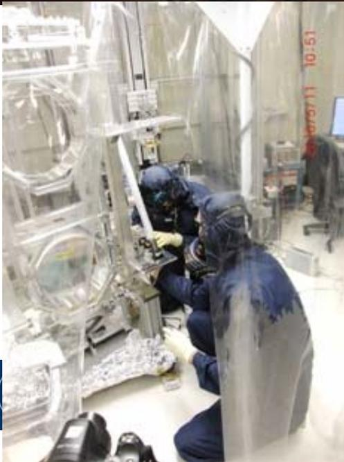
Building and installing quadruple suspension at LIGO Hanford site
