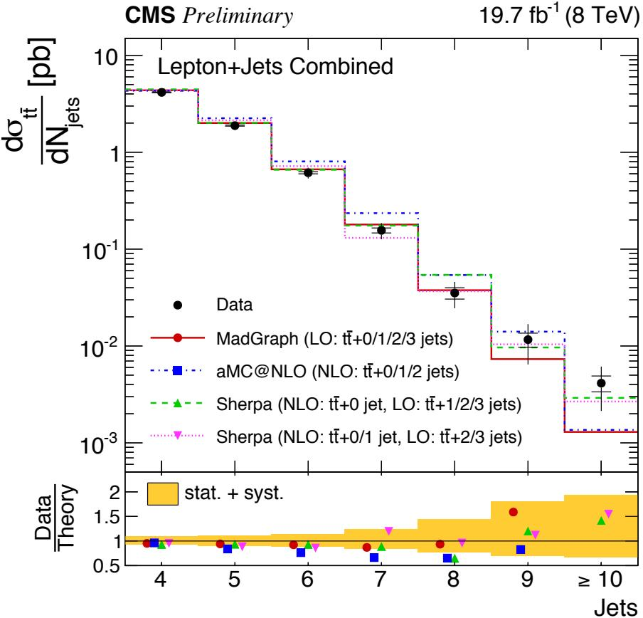
With the exception of MadGraph Q<sup>2</sup>/4 and MadGraph matching threshold of 10 GeV (down) most variations and generators agree with the data within the uncertainty
