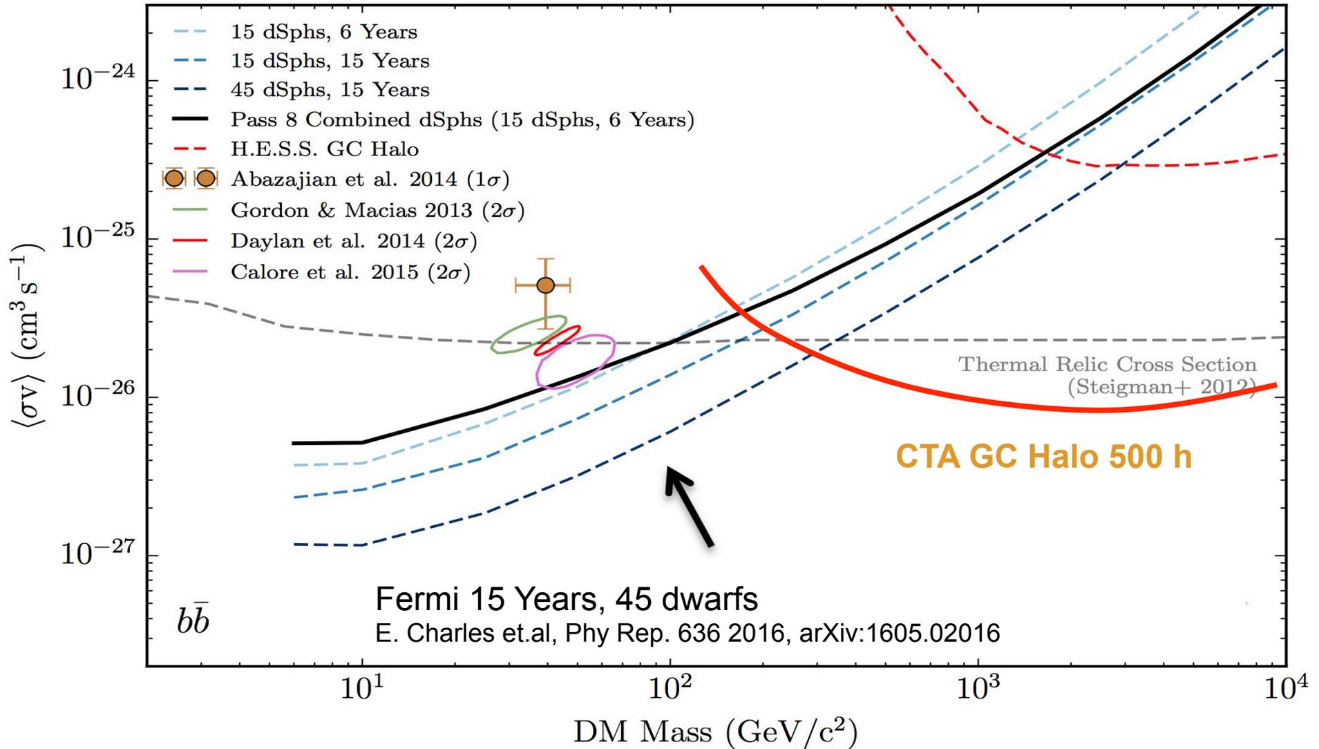
CTA sensitivity curve from Carr et al. 2015 500 hr, statistical only, NFW, 30 GeV threshold arXiv:1508.06128
