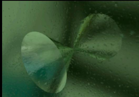
*Tracks are revealed as conical etch pits . Charge resolution  $\sim 0.05e$  .
