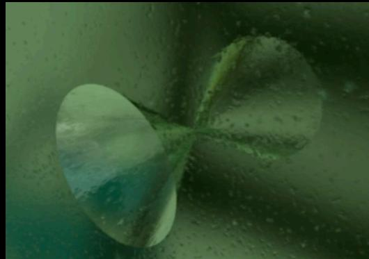
*Tracks are revealed as conical etch pits . Charge resolution  $\sim 0.05e$  . Spatial resolution  $\sim 10$  microns/pit – pointing to the IP*
