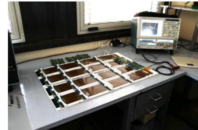
Testing Upstream Tracker 'flex cables'
