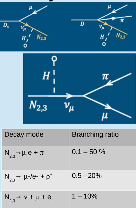
General experimental requirements to search for HS at beam dump experiment
