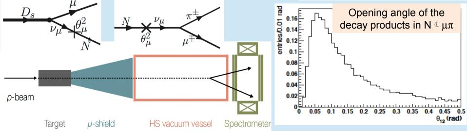
Detector must be placed close to the target to maximize geometrical acceptance. Effective (and "short") muon shield is the key element to reduce muon-induced backgrounds
