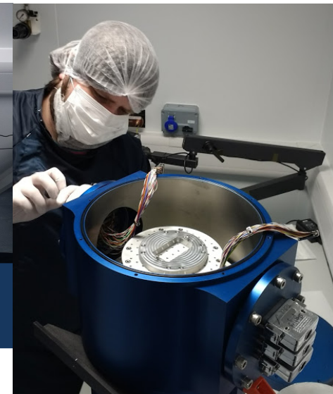
Installation of Teledyne e2v CCD in cryostat at Oxford
