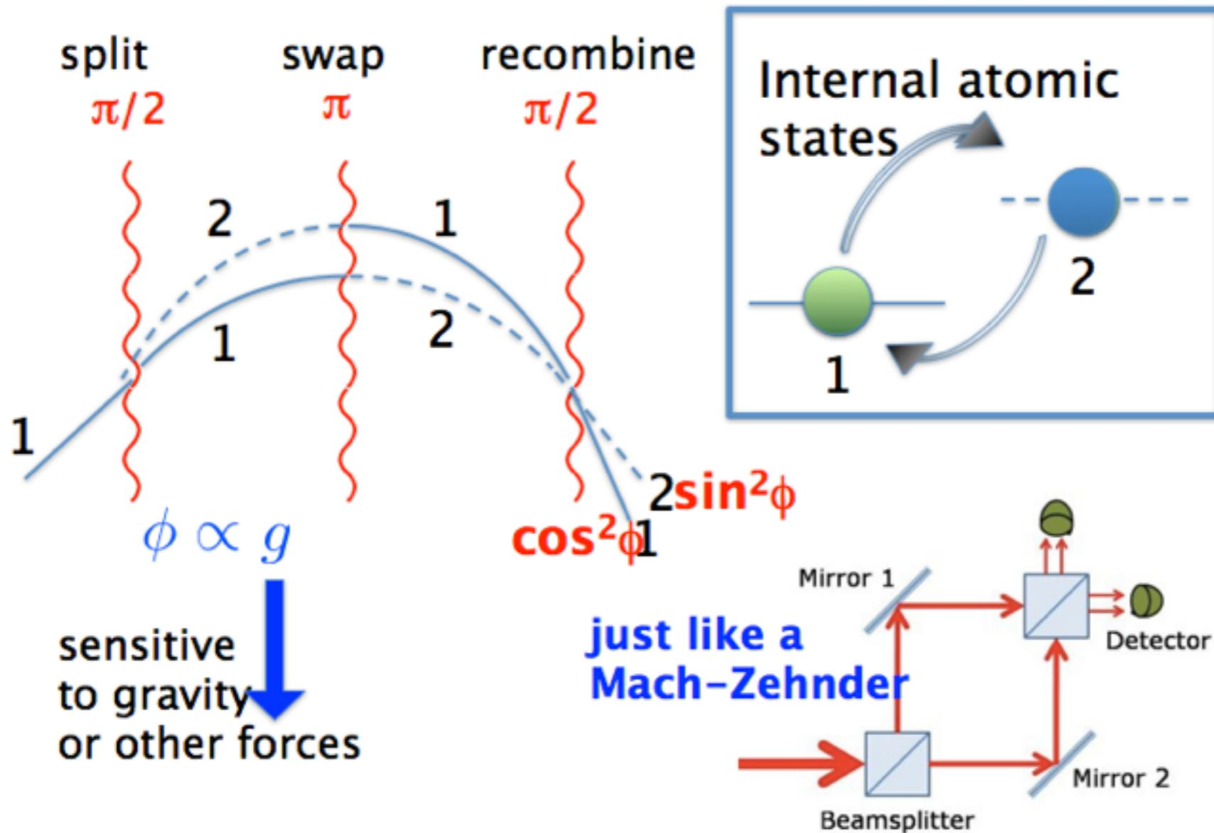
Raman interferometry uses a pair of counter-propagating laser beams, pulsed on three times, to split the atomic wave function, imprint a phase difference, and recombine the wave function.
