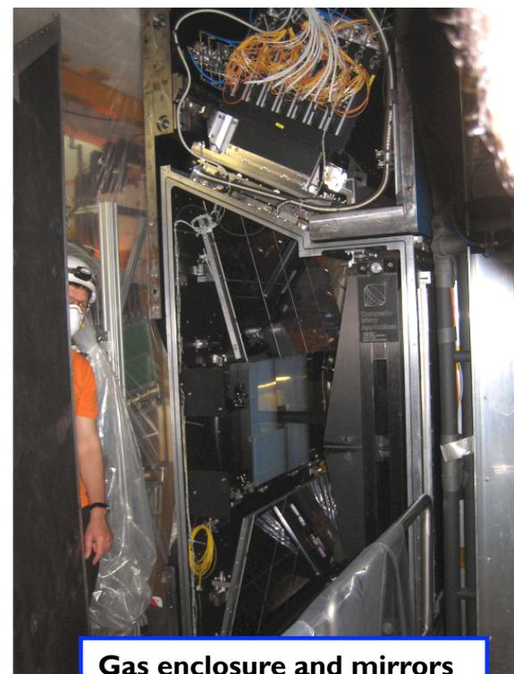
Gas enclosure and mirrors installed in LHCb pit
