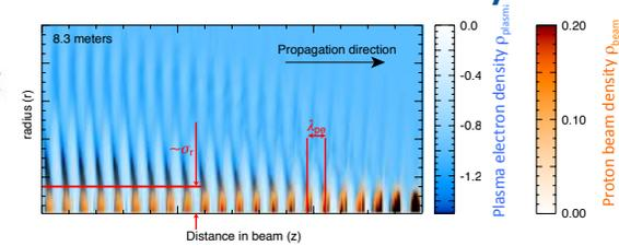
**Self-modulated proton bunch resonantly driving plasma wakefields.**
