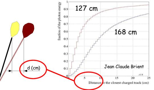
Energy deposited within "d" cm around a charged track
