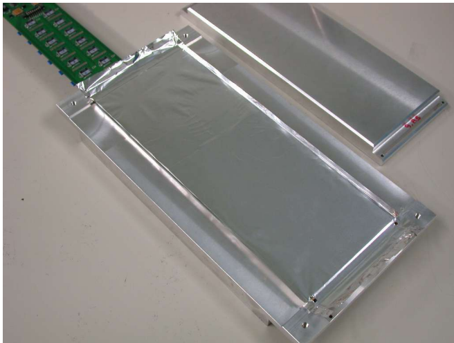
Wrap in aluminum foil – connect wafers to PCB ground (conductive EPO-TEK glue)
