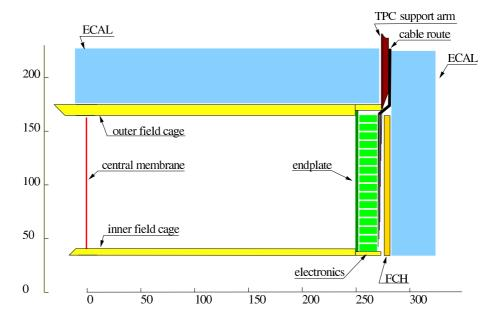
• Main mechanical parameters of the FCH for the
