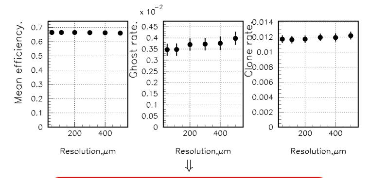
Small dependence on the drift-tube space resolution
