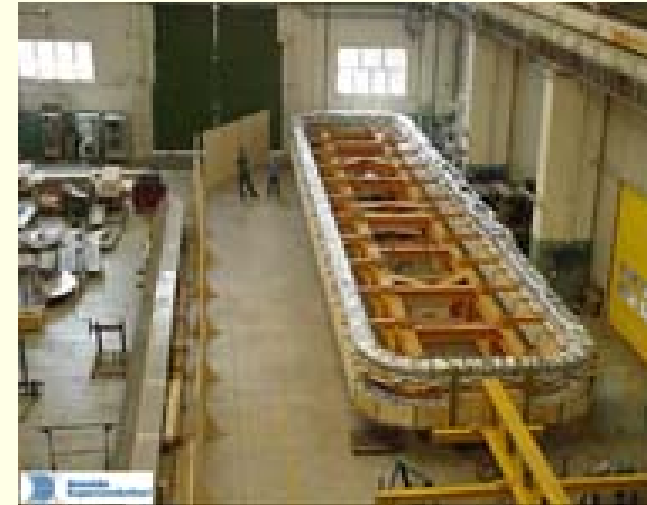
Central toroid under assembly
