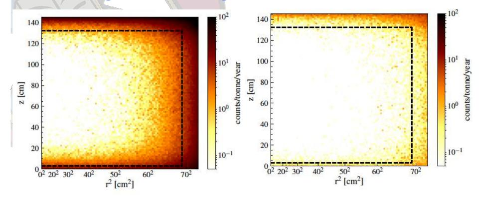
Single scatter nuclear recoil events in the LXe active volume before (left) and after (right) rejecting events in coincidence with veto system (LXe skin and the Outer Detector (OD).
