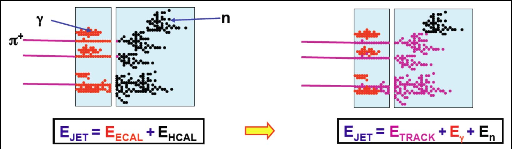
Detector must allow association of tracks with deposits in calorimeters
