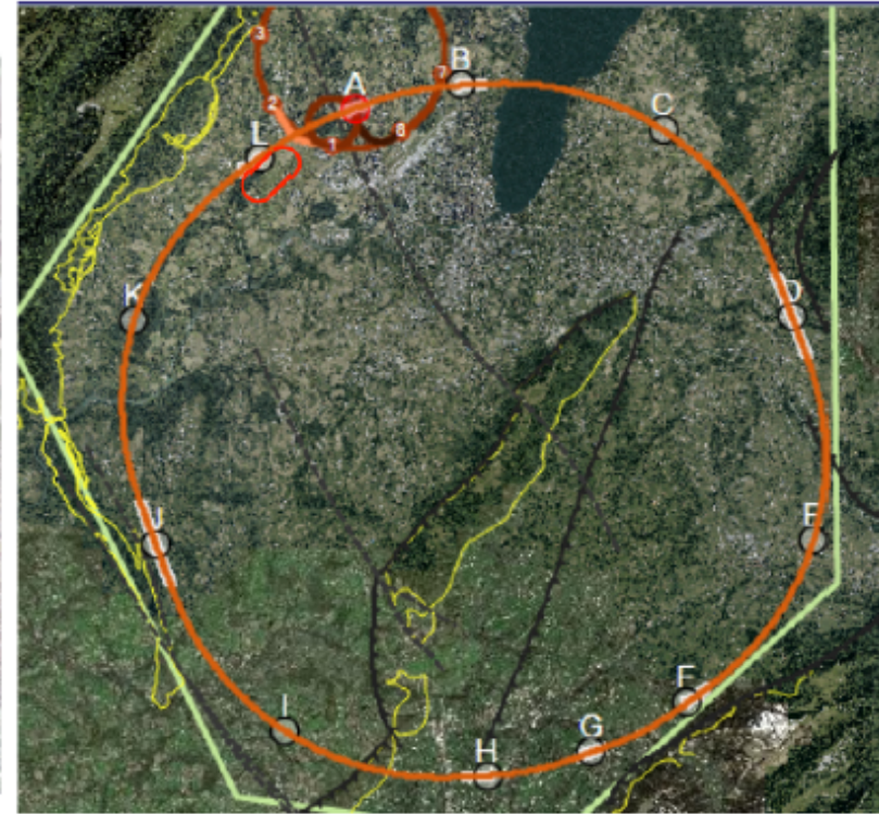
Figure 2: Possible locations of the ERL racetrack electron accelerator for the LHeC (left) and the FCC-he (right). The LHeC is shown to be tangential to Point 2 and Point 8. For Point 2 three sizes are drawn corresponding to a fraction of the LHC circumference of 1/3 (outer, default with E_e = 60 \text{ GeV} ), 1/4 (the size of the SPS, E_e = 56 \text{ GeV} ) and 1/5 (most inner track, E_e = 52 \text{ GeV} ). To the right one sees that the 8.9km default racetrack configuration appears to be rather small as compared to the 100 km ring of the FCC. Present considerations suggest that Point L may be preferred as the position of the ERL, while two GPDs would be located at A and G.
