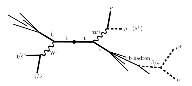
Measurement of the top-quark mass: m(t) is correlated with m(e/μ + J/ψ)
