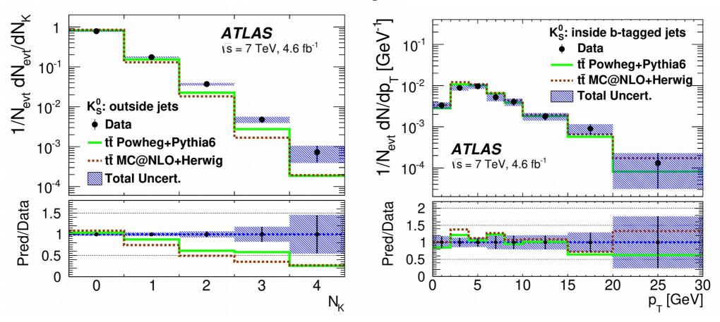
Unfolding to particle level applied to data. Unfolded distributions are compared to several MC generators and different MC tunes.
