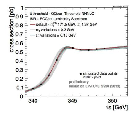
Multi-point threshold scan with 25 fb<sup>-1</sup> will determine  $m_t$  to 17 MeV (& also measure width & top-Yukawa coupling). At these energies RDP is not possible, but sufficient knowledge of  $E_{CM}$  will be achievable from reconstruction of WW, ZZ, Z $\gamma$  events. (True to say that this measurement is feasible for CLIC also.)
