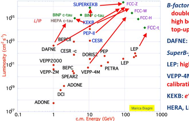
**B-factories:** KEKB & PEP-II: double-ring lepton colliders, high beam currents, top-up injection DAFNE: crab waist, double ring SuperB-factories, S-KEKB: low  $\beta_v^*$ LEP: high energy, SR effects VEPP-4M, LEP: precision energy calibration w. res. depolarisation KEKB: e<sup>+</sup> source HERA, LEP, RHIC: spin gymnastics
