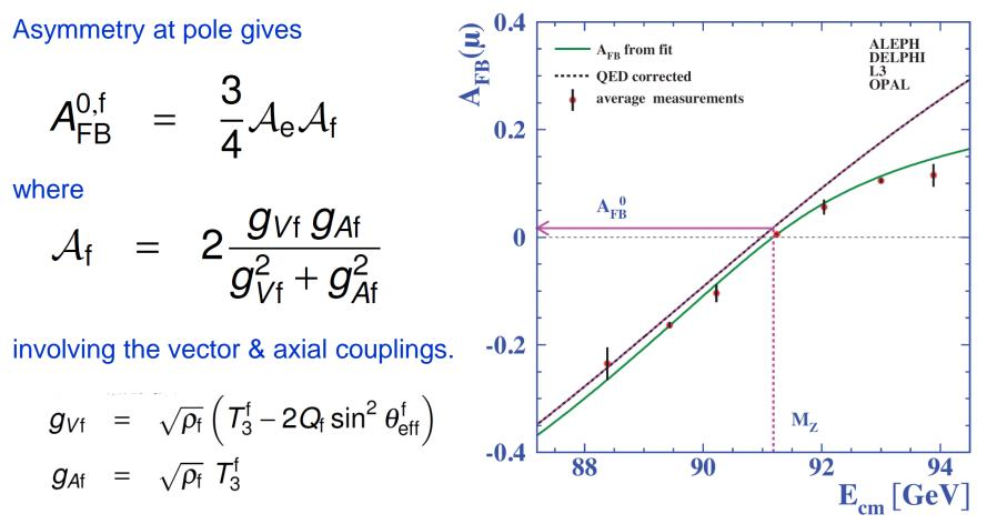
with  $\rho_f = 1$  in the limit of no radiative corrections (not a good approximation at LEP!). Off-peak asymmetries driven by  $\gamma$ -Z interference (FCC-ee sensitive to  $\alpha_{QED}(m_Z^2)$ ).
