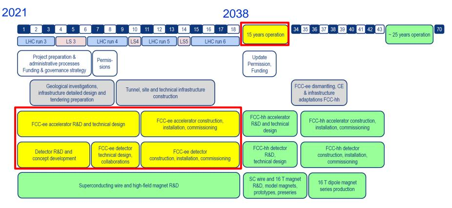
How much would it cost ? ~8 GCHF for tunnel (to be re-used by FCC-hh) ~4 GCHF for FCC-ee collider and injector (~17 GCHF for FCC-hh collider and injector – ouch !)
