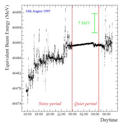
Found to be due to magnets being 'tickled' by current on beam pipe from passing trains.
