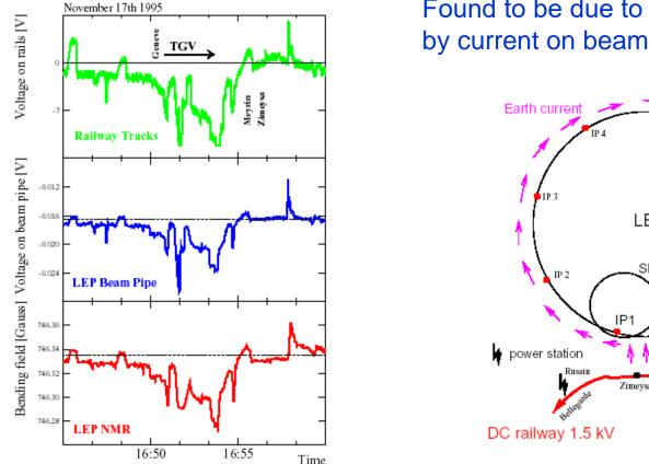
Found to be due to magnets being 'tickled' by current on beam pipe from passing trains.
