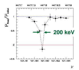
Monitor polarisation with Compton scattering from laser whilst exciting beam with transverse oscillating B field. Find frequency at which depol<sup>n</sup> occurs.
